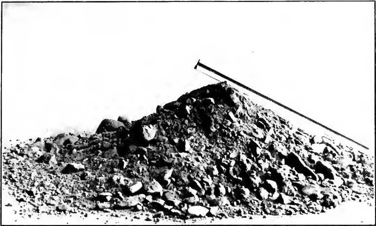
FIG. 6.—COMBINED COARSE AND FINE MATERIALS, MIXED IN EQUAL PARTS OF EACH.
